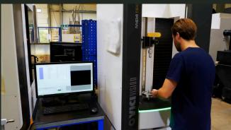
The VICIVISION machines are strategically positioned on the shopfloor, next to machine tools. Operators can quickly inspect freshly-made components by running preprogrammed routines at the press of a button.
