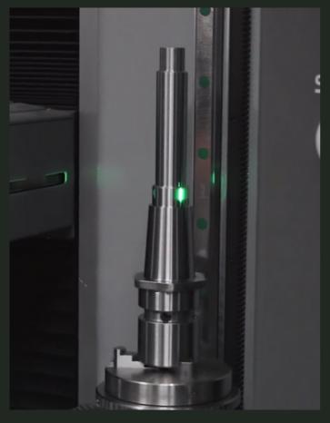
Unimaq invested in a <u>M609 optical part</u> <u>measurement machine</u> from VICIVISION UK to speed up their inspection processes and ensure the high-levels of accuracy required.
