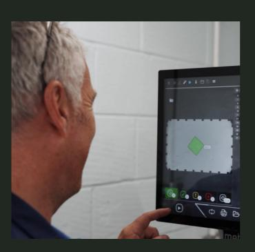
**56** You can put 15 components on the Metrios machine at once and it'll measure them in 4.5 seconds.
