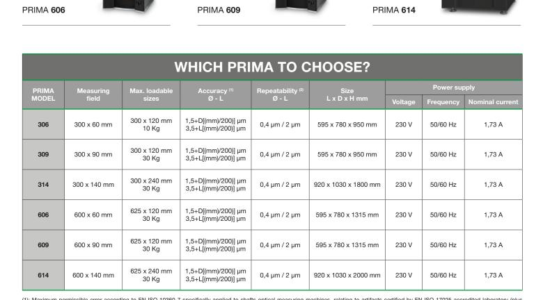
(1): Maximum permissible error according to EN ISO 10360-7 specifically applied to shafts optical measuring machines, relating to artifacts certified by EN ISO 17025 accredited laboratory (plus uncertainty of calibration masters U(d): 0.5 µm and U(l): 1 µm), steel made, ground surfaces and standard shape. Environment condition 20+/-0.5°C, max gradient 0.5 K/h. Uncertainty esti considering a coverage range K=2 corresponding to a confidence level of about 95%.
